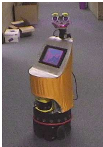
Figure 1: Side view of Flo, the robot. The robot is equipped with a touch-sensitive display, a laser range finder, an array of 16 sonar sensors, and two on-board PCs.
